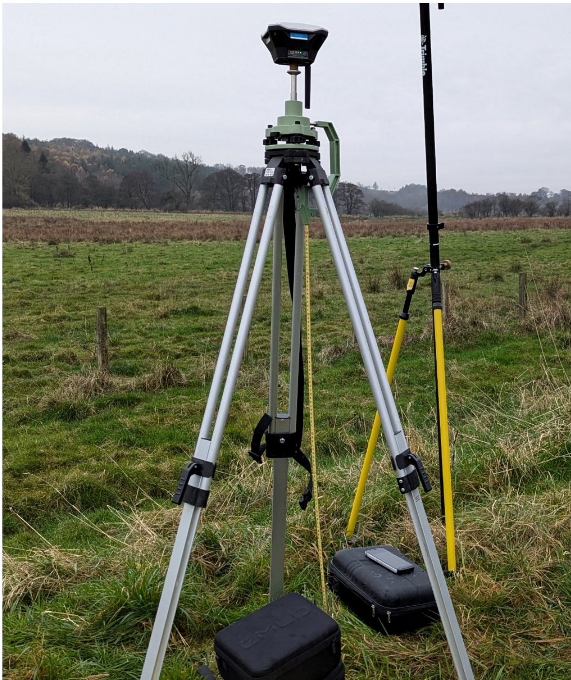
Figure 47 - Emlid RS+ GNSS base mounted on SECO 5301 tripod showing inbuilt tape measure
