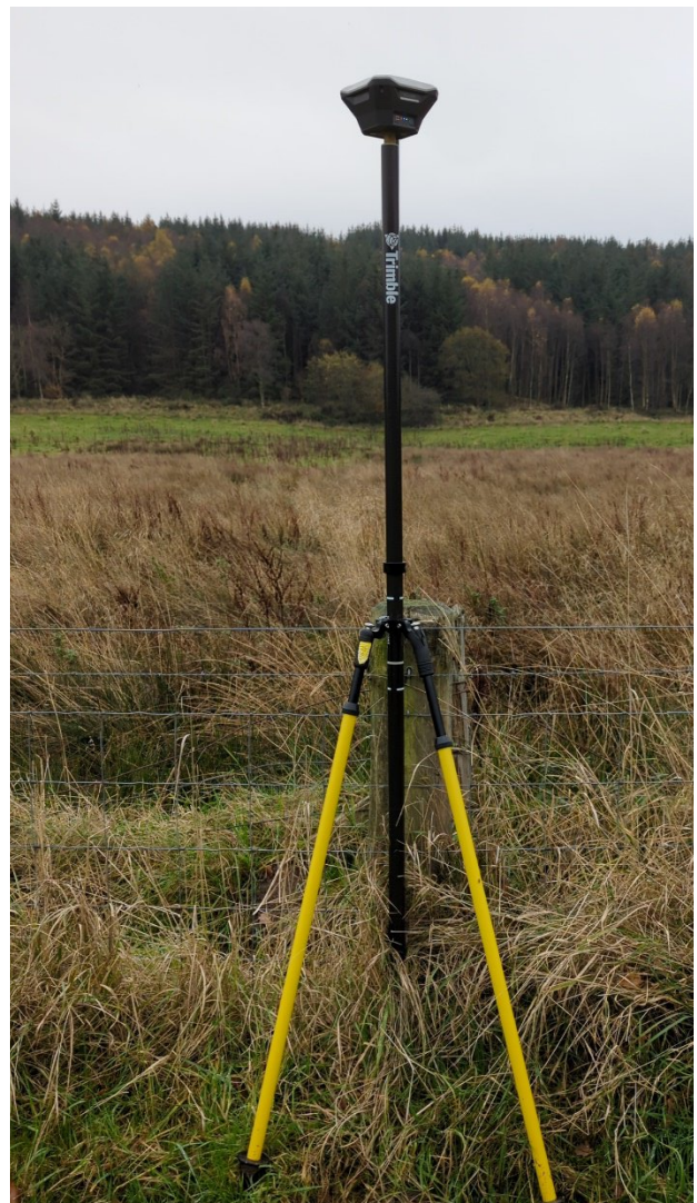
Figure 49 - Emlid GNSS receiver capturing GCP 49 with Melloch Woods in background
