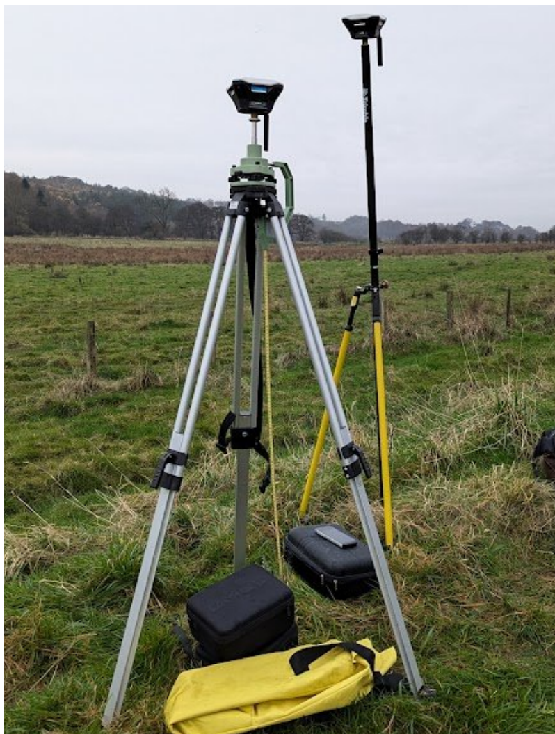
Figure 6 - Emlid RS+ GNSS base (left) and receiver (right)
