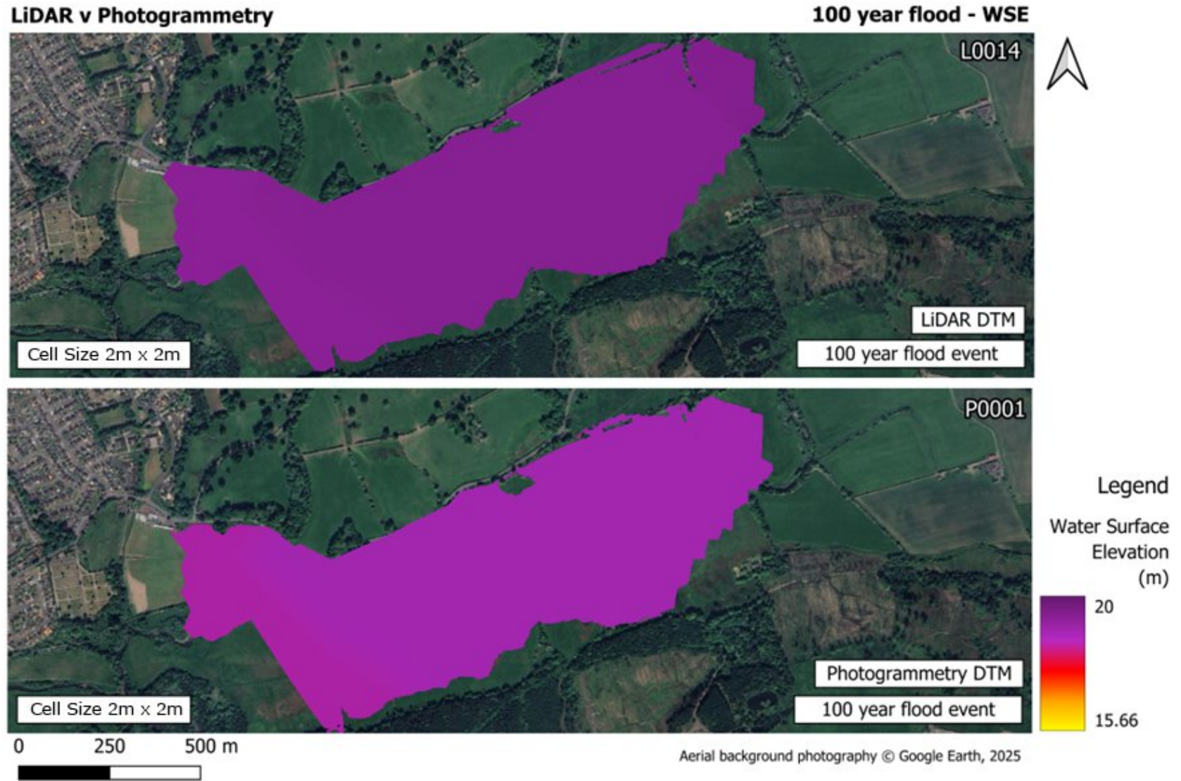
Figure 24 - 2D (unsteady) model comparing WSE results for 100-year flood
