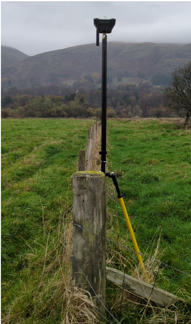
Figure 48 - Emlid GNSS receiver capturing GCP 01 with Ochil Hills in background
