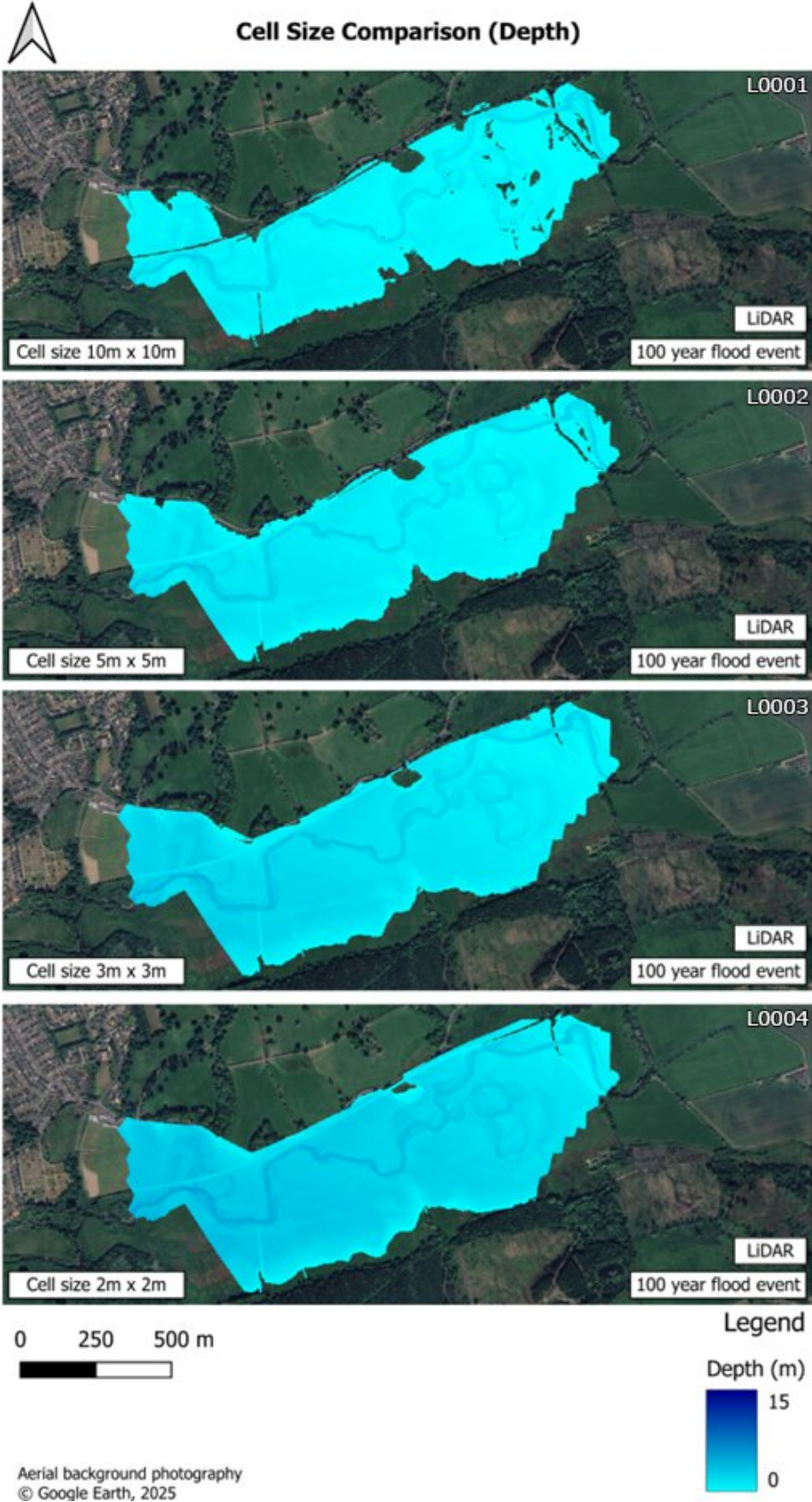
Figure 20 showing large differences in extent of flood and depth of water between different cell sizes.
